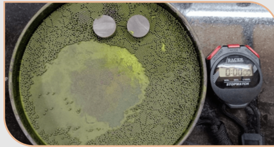
DYE PENETRATION TEST
